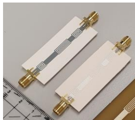
RLC RF Zinc resonators printed on paper
