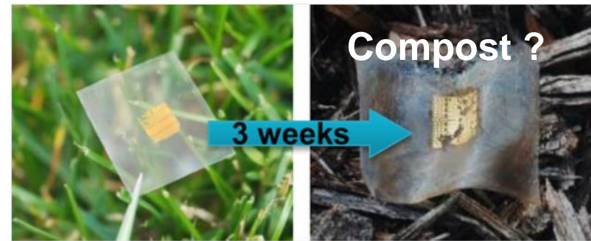
Biodegradable silicon electronics demonstrated
